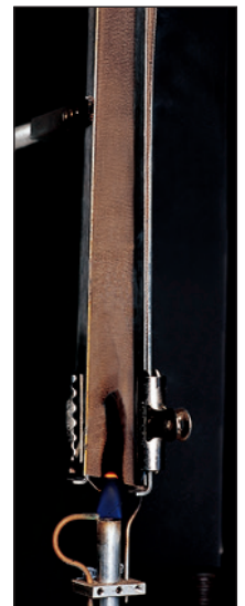
Vertical flame test on Westex UltraSoft® fabric
